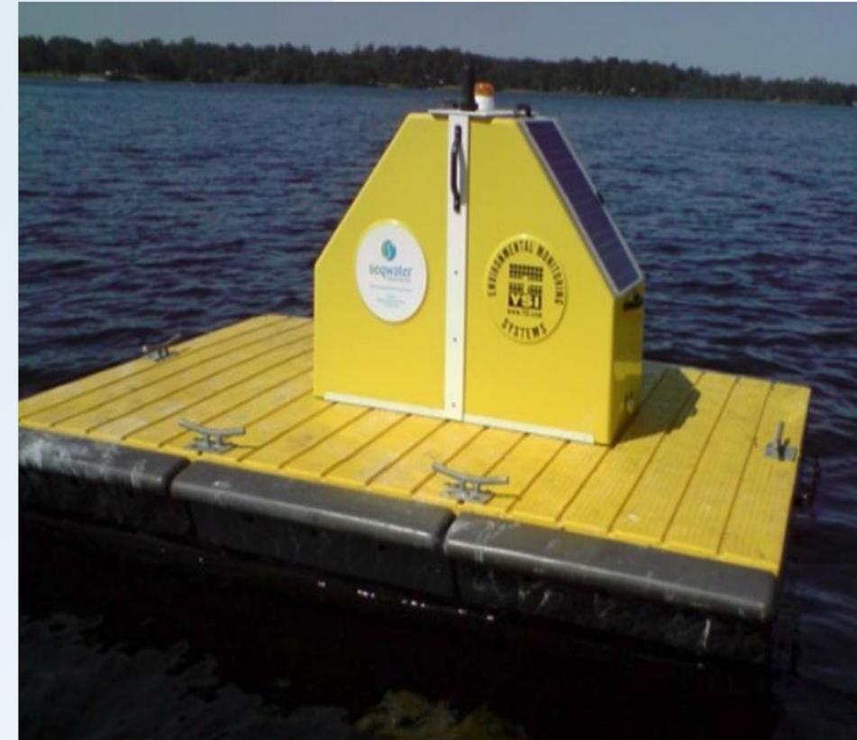
General scheme of the automatic water quality-monitoring station and the buoy containing the vertical profiler
