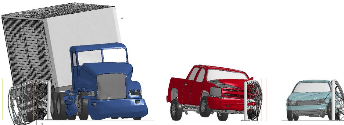
**Figure 1 – Simulation of TL5 according to MASH (respectively 36000V, 2270P and 1100C)**
