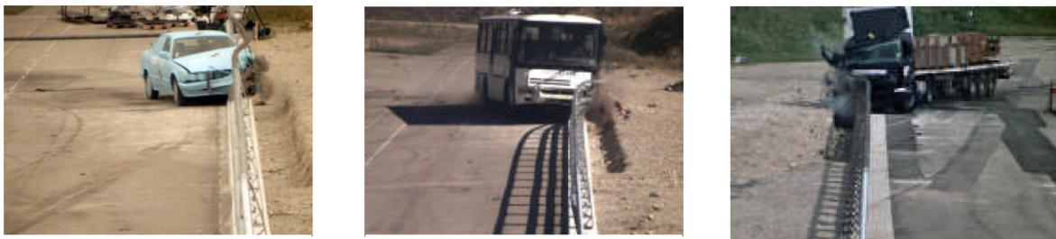
Figure 3 – Comparison between crash test and numerical simulation (DOLRE H241 – TB51 according EN1317)
