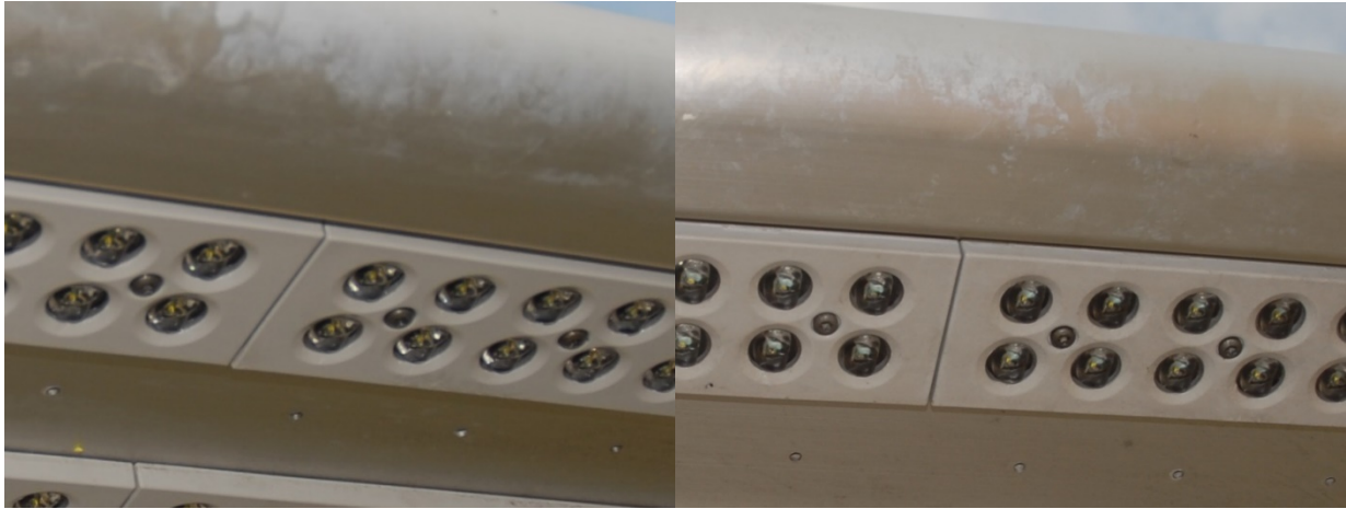
Figure 57. Before and after cleaning pictures. There is no visual difference.
