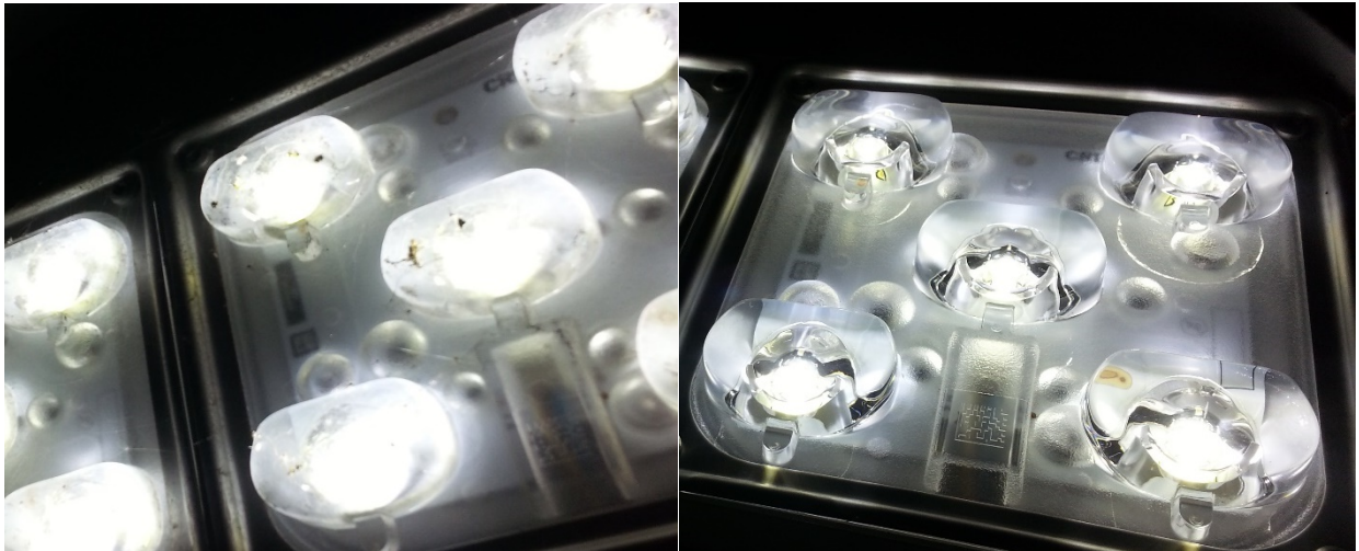
Figure 56: Design L, large individual molded plastic optics: dirty (left) and clean (right).
