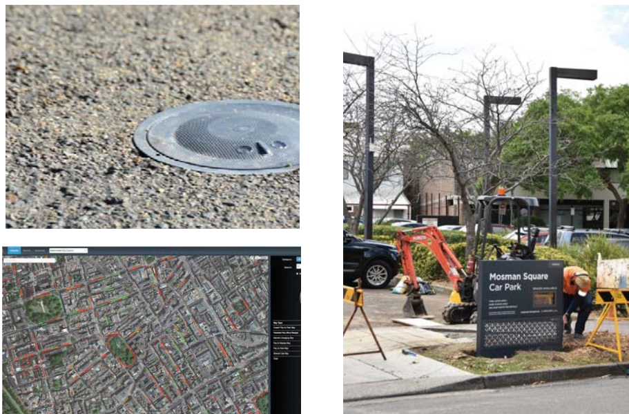
Figure 1: Top Left a smart parking in ground sensor. Bottom Left the Smart Parking Dashboard showing sensor location and occupancy. Right the installation of an electronic parking sign connected to the sensors.
