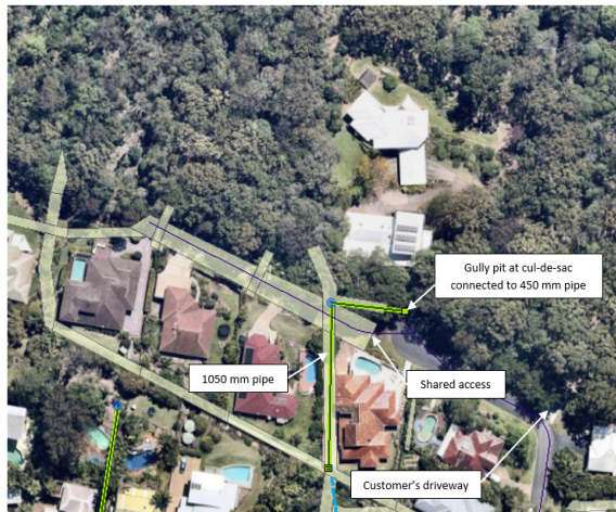
Figure 2: Stormwater network layout (Sunshine Coast Council, 2018)
