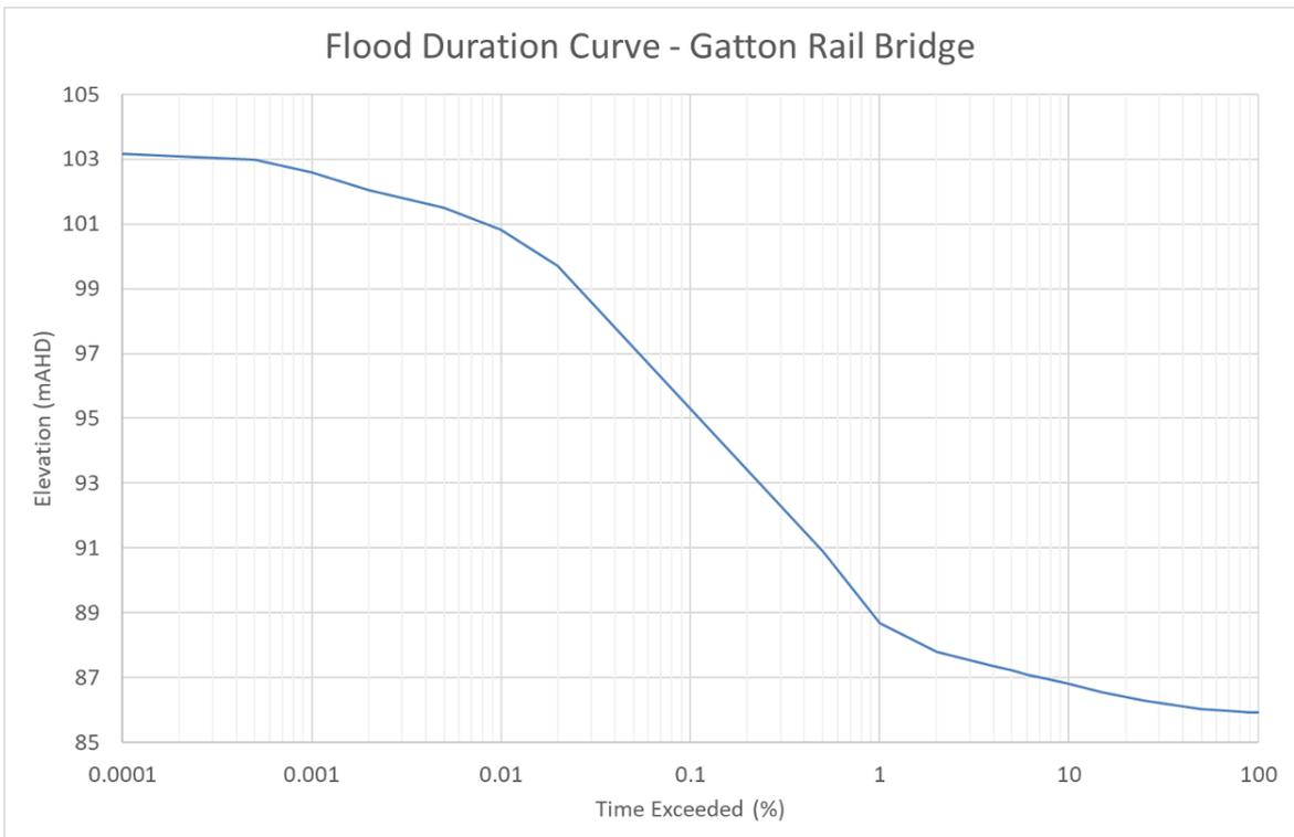
Figure 5: Flood level duration curve at Gatton Rail Bridge generated from model results
