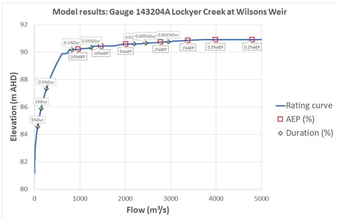
Figure 3: Rating curve at Gauge 143204A generated from model results
