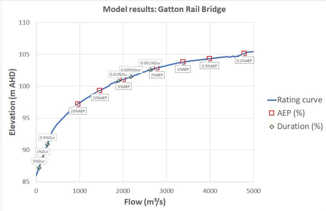
Figure 4: Model results at Gatton Rail Bridge, showing rating curve, AEP and duration
