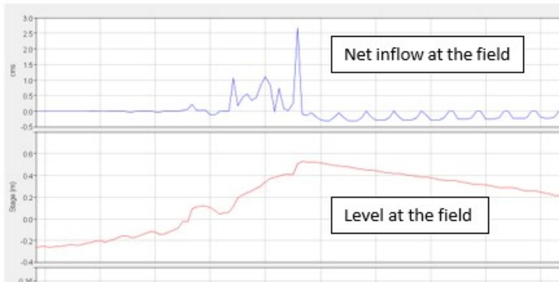
**Figure 9: Model behaviour at cane field, showing discharge to the cane drains during low tides following a major rainfall event**
