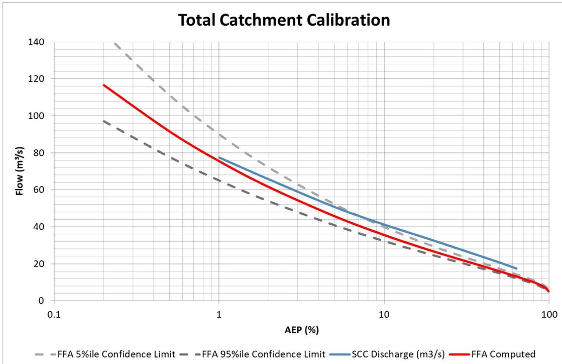
**Figure 10: Example of flood frequency analysis of model results and comparison with SCC Discharge Estimation Tool**
