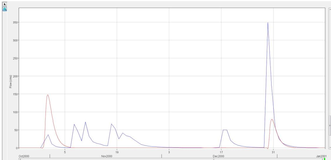
**Figure 15: Comparison of observed (blue) flows and modelled (red) flows at a river gauge**
