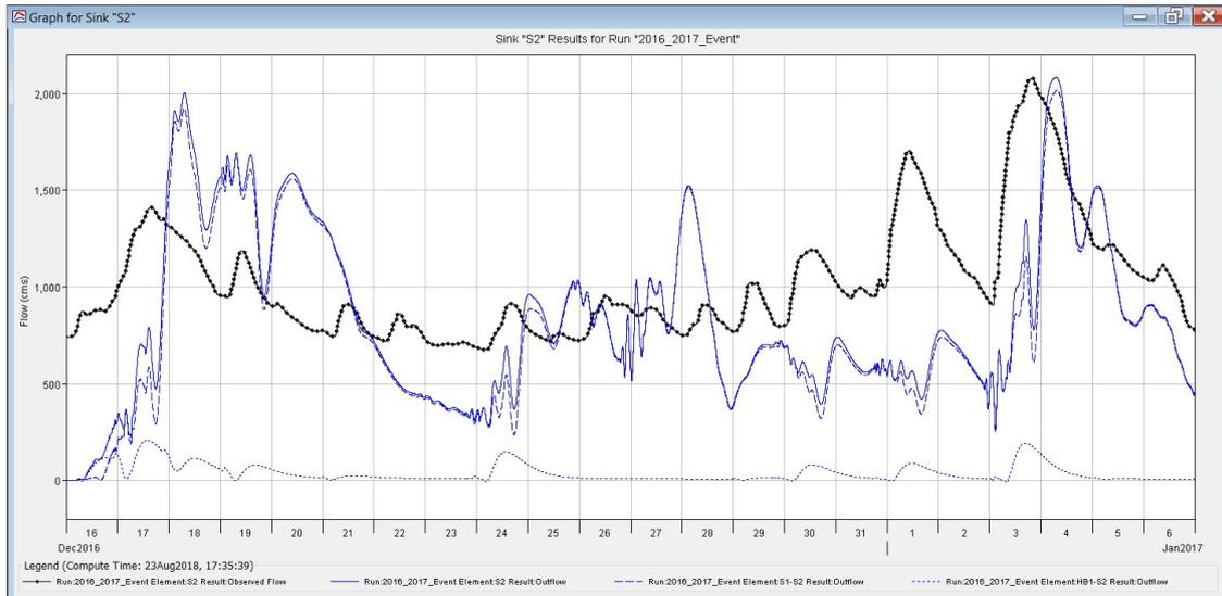
**Figure 13: PNG Study, Calibration at lowland catchment (observed data in black, modelled data in blue)**
