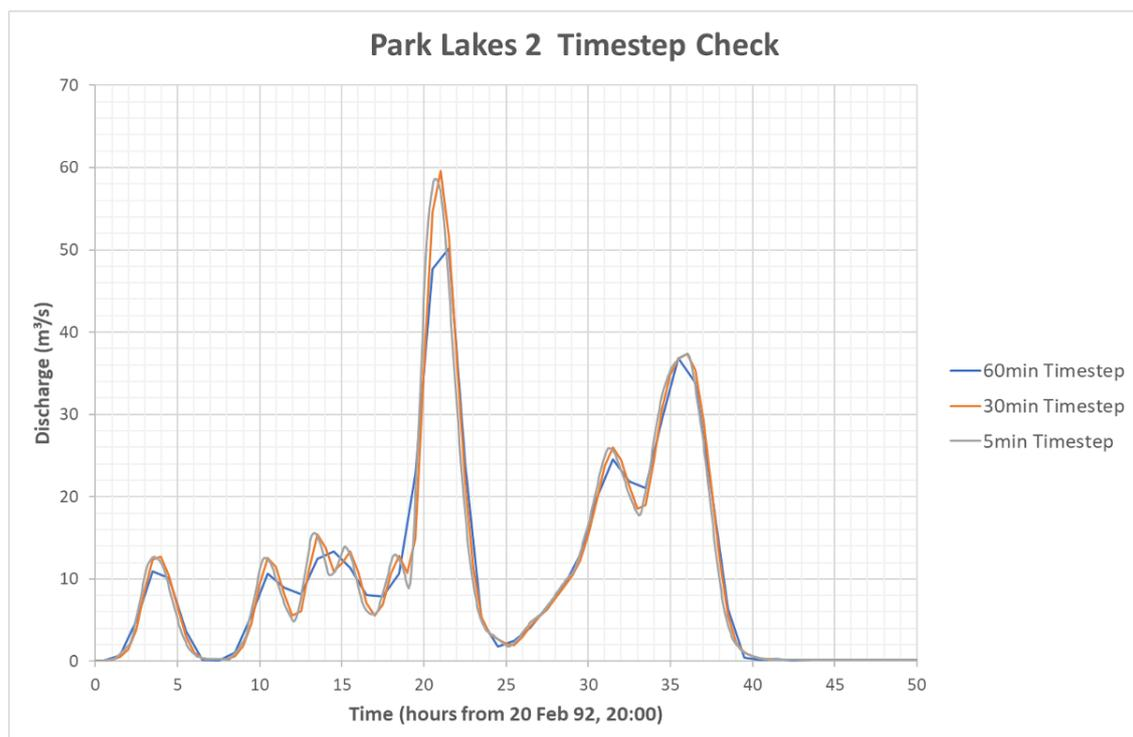
**Figure 8: Hydrographs from sensitivity tests using different timesteps**
