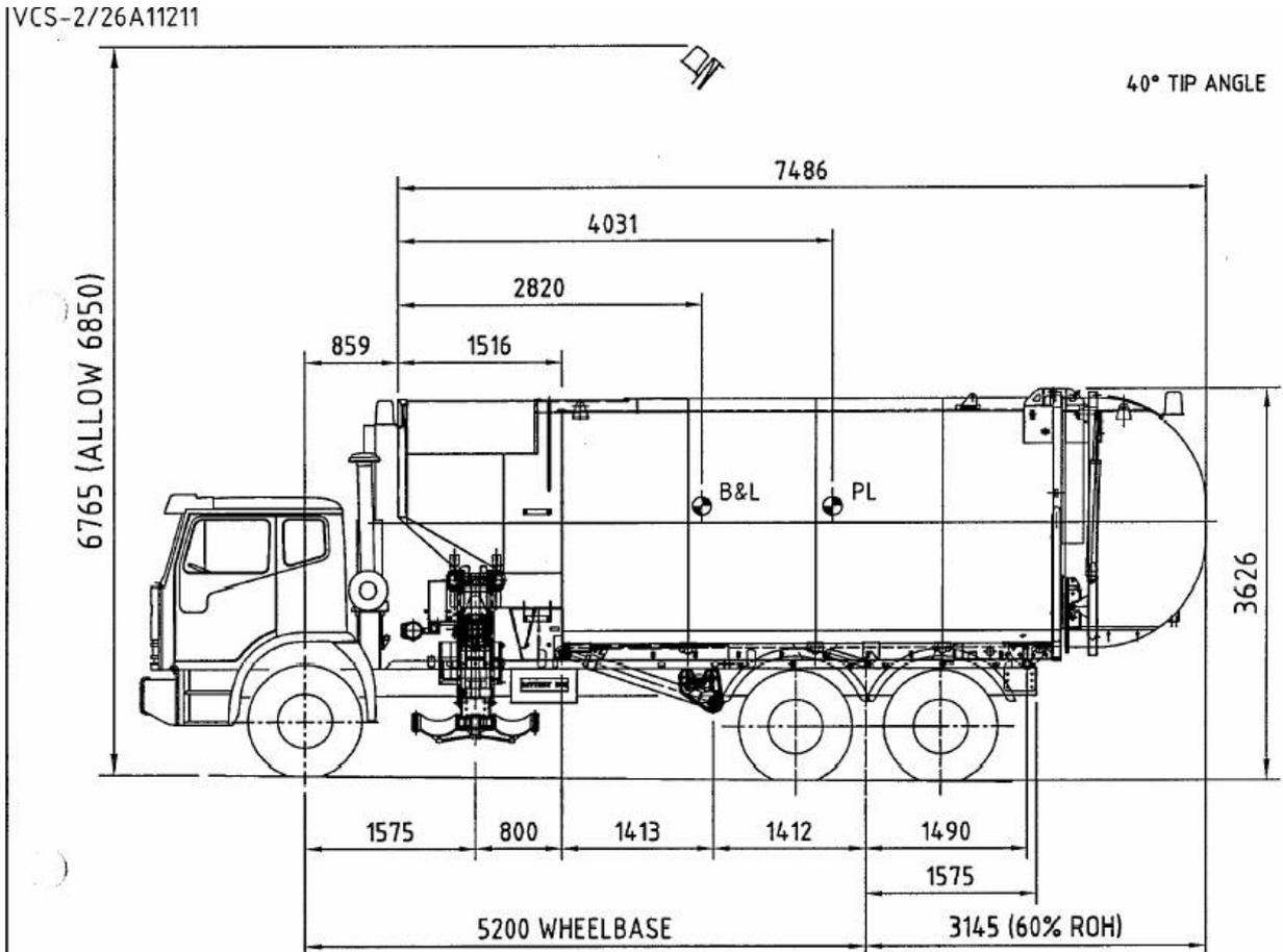
BASED ON A DENSITY OF 145kg/m<sup>3</sup> FOR RECYCLABLES, THE MAXIMUM ACHIEVABLE PAYLOAD FOR 29m<sup>3</sup> IS 4205KG.
